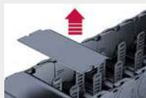
Detach the cover from the chain link
