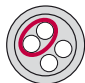
Element shield continuous bending hi-flex, in-plated braided copper shield with the option of foil shield – see type/design
