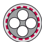
Overall shield continuous bending hi-flex, tin-plated copper braiding for smallest bend radii Coverage: approx. 80 %
