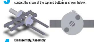
Rotate the entire ECCT tool until the top and bottom posts
